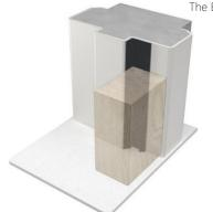
The Batwing acoustic and smoke seal minimises the opening and closing resistance of the door leaf.
