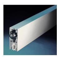
An aluminium-based drop seal for acoustic, smoke and energy containment. It features a high efficiency mechanism which lifts the seal clear of the floor as soon as the door is opened by a few millimetres.
