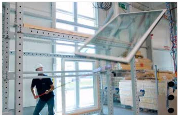
All our windows are drop tested, this tests the capability of the ironmongery to stop the window falling from the facade should any piece of ironmongery fail. VELFAC windows are proven to be safe and secure.
