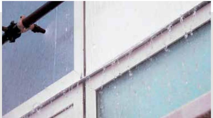
Window façade exposed to CWCT water load test. Water nozzles are located directly in front of the façade and water pumps with a flow rate of at least 3.4 litres/m<sup>2</sup>/minute.
