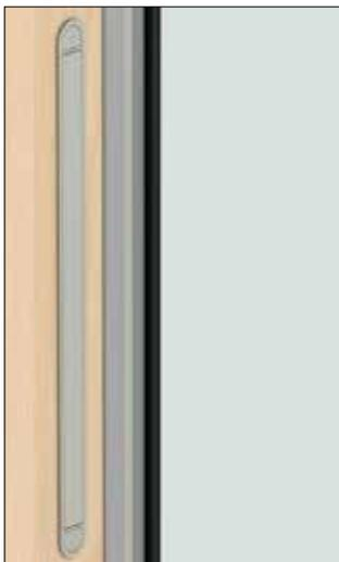
**Click vent.** Anodized surface finish. Fully concealed. Free ventilation opening in elements with 24mm glazing: 4000mm<sup>2</sup>. Free ventilation opening in elements with 48mm glazing: 3000mm<sup>2</sup>. For the equivalent free opening, please refer to our website.
