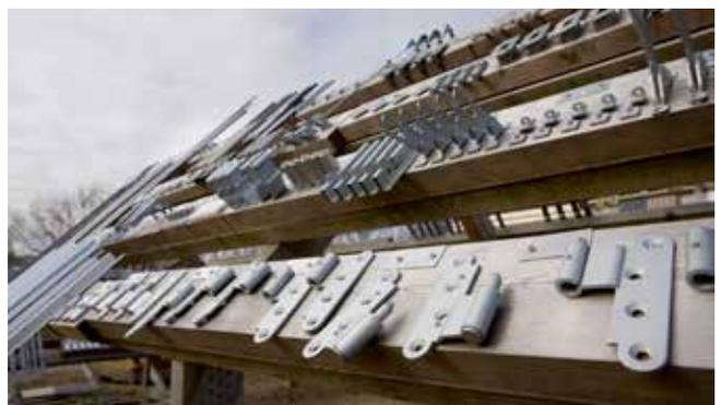
Our R&D Department develops the majority of VELFAC ironmongery to ensure it is ideally suited to the style and function of the VELFAC system, and all items are regularly tested both by VELFAC and by independent testing bodies. Here, VELFAC ironmongery is exposed to salt-laden winds and coastal weather conditions.
