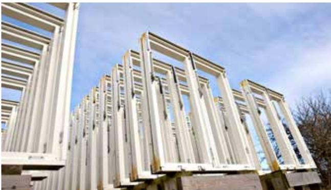
VELFAC frames exposed to high winds, rain and sun. This tests the durability of different surface treatments.
