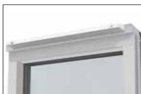
**Acoustic trickle vent.** The vent is machined into a timber packer with an external aluminium profile in the same colour as the door frame. Documentation on air flow can be requested. Achieves a sound reduction value of  $D_{n,e,w}$  40 dB.
