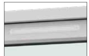
**Click vent.** For outward opening doors only. Natural anodised surface finish. Free ventilation opening 4000mm<sup>2</sup>. Documentation on air flow can be requested.
