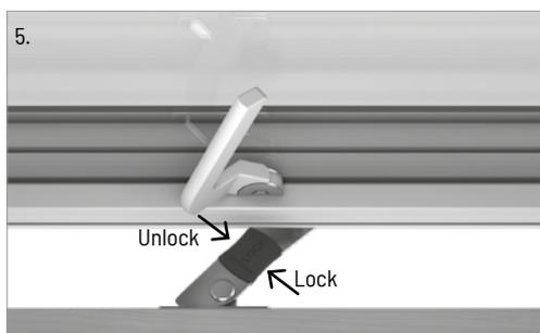
**Locked in ventilation position.** Lock the restrictor by pushing the red plate until a click is heard.
