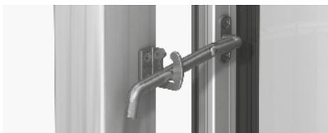
> **The PN-fitting** makes it difficult for unwanted guests to enter if the window is open. When opening the window, the arm is lifted and re-engaged when the required opening is achieved. The arm is raised to a vertical position to disengage, allowing the sash to open fully.
