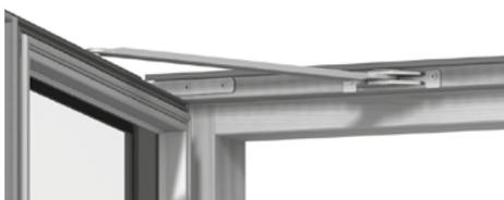
> **The friction arm** will retain the open window in any ventilation position under normal weather conditions. If it is really windy the ventilation position in the handle is to be used instead (see p. 18). The friction arms are adjusted by the factory to fit the size of the window. If the window opens too tight or too loose, the friction arm may be adjusted (see more by the relevant type of window).
