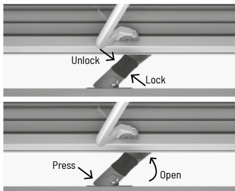
> **The opening restrictor** automatically engages when the sash is opened to approximately 10cm.
