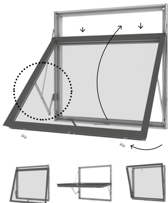
The window opens by turning the handle to a vertical position and pushing the sash outwards until the restrictor engages at an opening of 5-10cm. Notice if your window has a hinged or a straight reversal bracket.
