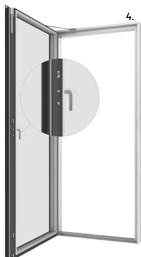
**Handle operated brake.** The casement door might have a handle operated brake, that can hold the door in any open position from approx. 10-85°. The brake is activated by opening the door to the desired position and turning the handle down to the vertical position (4).
