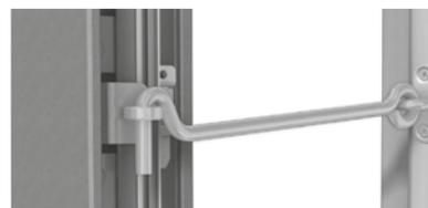
> **Window stay.** The arm is fitted to the wood frame and when used, is hooked into an eyelet on the sash to achieve an opening of approximately 130mm.
