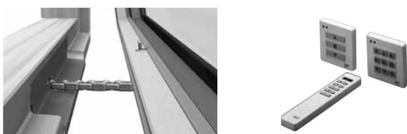
> **Remote operation** is operated via a panel on the wall - or a remote control. The window is opened with the arrow-up button, and closed with the arrow-down button. The remote comes in two versions: The window moves while the button is pressed down - or by one short press and stop with the middle button. The metal chain of the remote operation should be kept clean.
