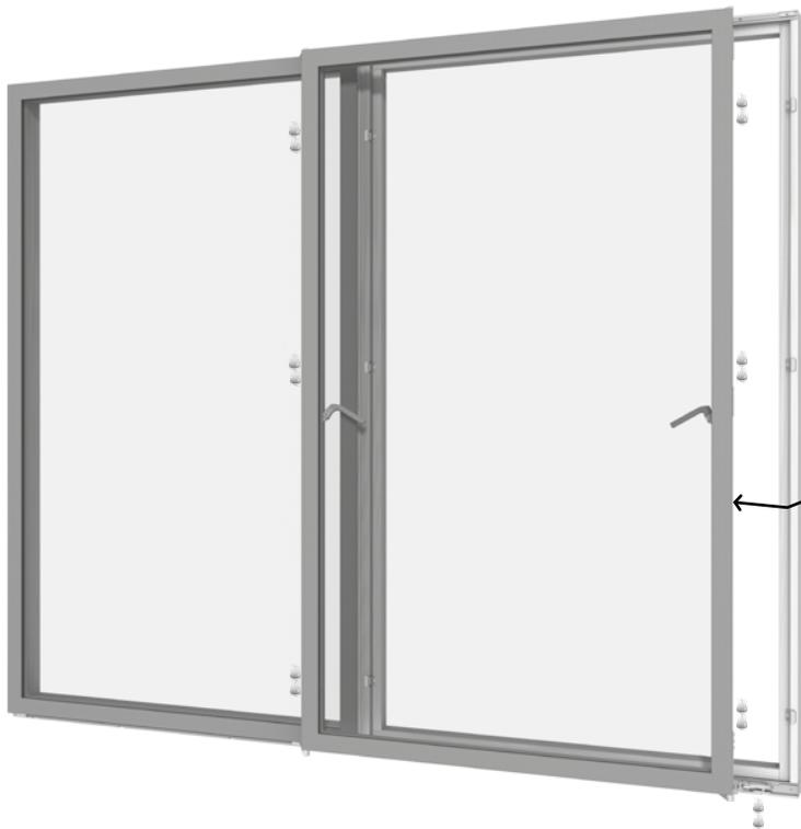
The sliding door is opened by turning the handles at the sides of the door leaf to a horizontal position. The door is then pushed outwards approximately 10cm and slid across. The door is closed by sliding across and pulling back toward the frame. The handles are then turned back to a vertical position.
