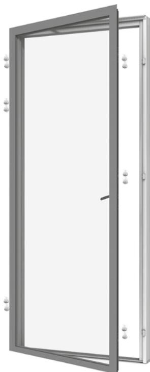
The casement door is opened by turning the handle to a horizontal position and pushing the door leaf outwards. The door opens to 90° and is equipped with a friction arm which allows it to be held in any position between closed and fully open. Doors can be fitted with a hinge to allow 180° opening but then cannot be fitted with a friction arm.
